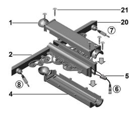
• Attaching the Lamp Support Assembly to the Base & Post Assembly: Lay the assembled lamp post and base down on the floor to thread the power wire (10) through the lamp base and lamp post. After drawing out the power wire's connector through the top of the lamp post and holding it securely, set the lamp post upright on its base, letting the power wire hang over the top.
